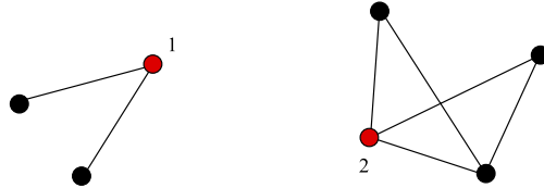
Figure 1: Example of the clustering coefficient calculation. Node 1 has a clustering coefficient of 0, its two neighbours are not connected. The clustering coefficient of node 2 evaluates to C_2=2/3 with y=2 and z=3 .
